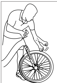
Fig. 17: Strike the wheel in a downward motion.
