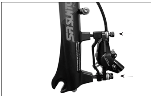
Fig. 14: Attach the front brake caliper.
