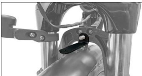
Fig. 21: Install L shaped bracket and attach end nut.
