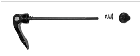
Fig. 15a: Remove end nut and first spring.
