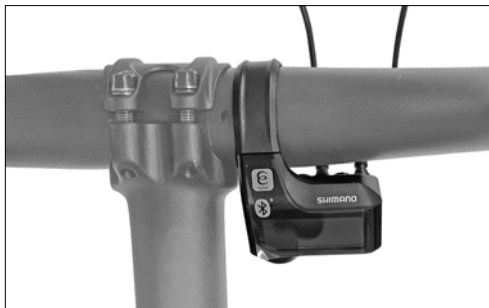
Fig. 11b: Clamp the display screen to the bars.
