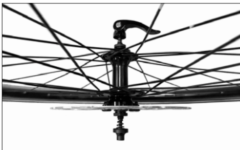
Fig. 15b: Slide skewer into wheel and replace nut.
