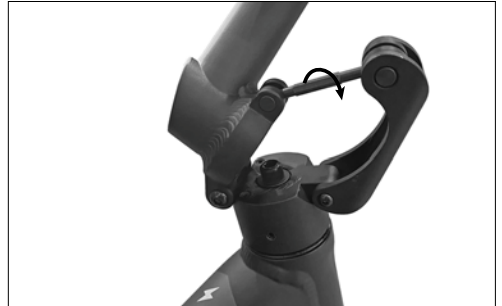
Fig. 51: Turn barrel adjuster to tighten quick release
