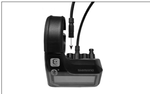
Fig. 11a: Plug the power cable into the display.
